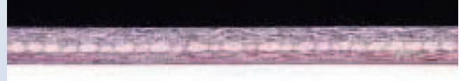
Print through effect from the 65 mils of skin in the open molded panel.
